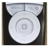
**4 Arrows**: The **4 arrow** buttons are to move up, down, right, and left in a menu when navigating the screen.
