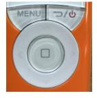
**OK**: The **OK** button is the round button in the centre with the square on it. This is the button to use when confirming an operation.
